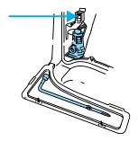
7. Position the jack according to the following guides and turn the jack handle clockwise until the tire is a maximum of 25 mm (1 inch) off the ground.
